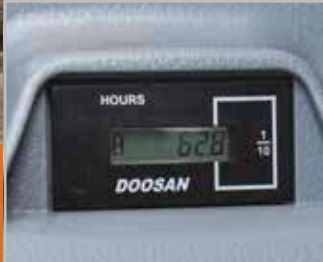
Hour meter (from ground level)
