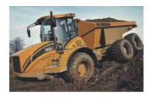
surfaces, due to the oscillated and hydraulic stabilized pivot joint. Combined with electronically controlled suspension and level control on the front axle, the result is a very high operator comfort.
