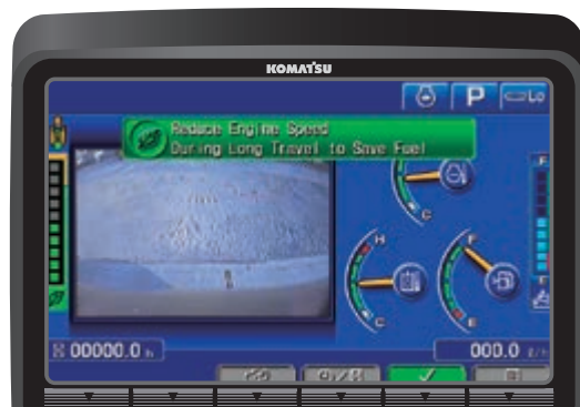
Improved monitoring system with rear-view camera image on the default screen. Eco gauge, eco guidance and fuel consumption gauge help to further reduce consumption.
