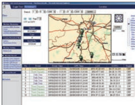
Machine tracking during transport - When your machine is transported, KOMTRAX™ sends travel messages to the web site or by e-mail to inform you of its progress, and confirms when it reaches its destination.
