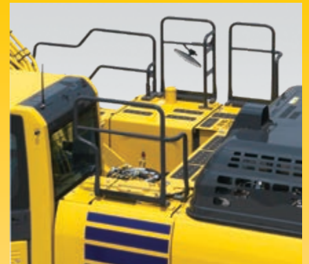
Hand rails and anti-slip plates
