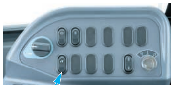
Dual mode engine power selection switch
